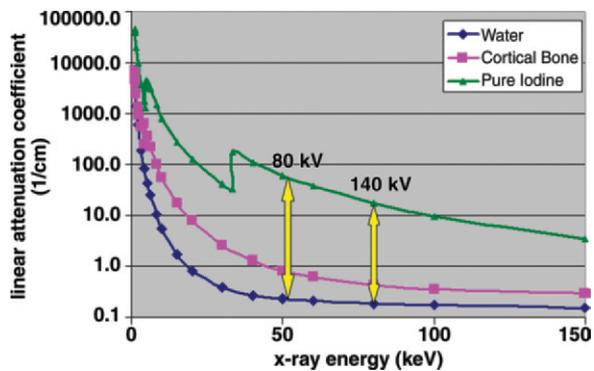
**Figure 4.** Graph shows the linear attenuation coefficients of iodine, cortical bone, and water, which are plotted as a function of x-ray energy. Note the difference between the linear attenuation coefficients of iodine (top curve) and water (bottom curve) at the mean energy of a typical 80-kV (long arrow) and 140-kV (short arrow) x-ray beam.
