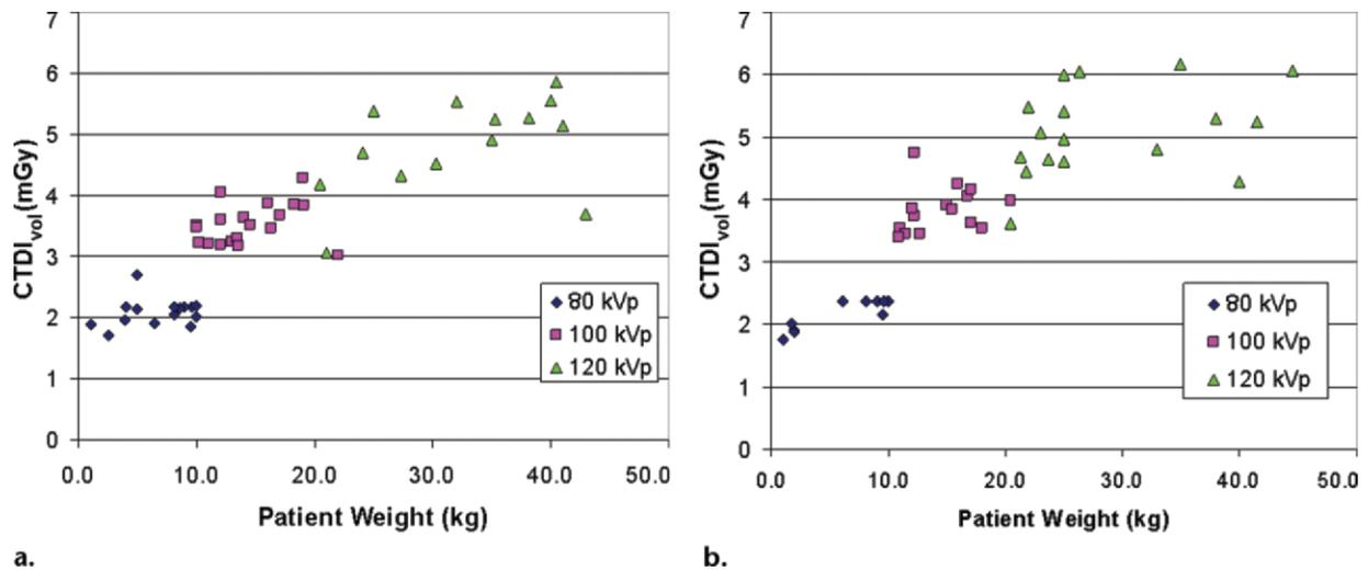
**a.** **b.** **Figure 10.** Graph shows the distribution of  $CTDI_{vol}$  as a function of patient weight on the basis of the technique charts for pediatric chest (**a**) and abdominopelvic (**b**) CT examinations. The  $CTDI_{vol}$  value is based on a 32-cm CTDI phantom.
