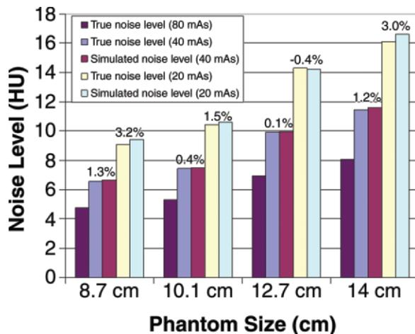
**Figure 8.** Graph shows the effectiveness of the noise insertion tool on four acrylic cylindrical phantoms (8.7 cm, 10.1 cm, 12.7 cm, and 14 cm). Two simulated dose levels (50% and 25% of the original doses) were included, and the noise levels in the simulated images were compared with those in the images acquired directly from the CT scanner.
