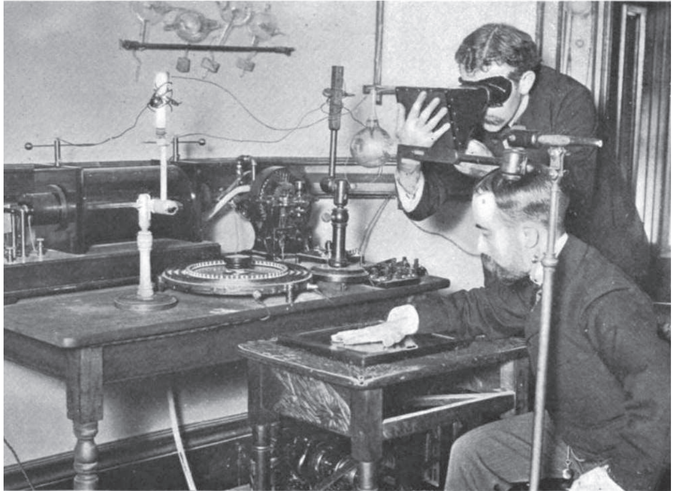
Photo of experimenters taking an x-ray with an early Crookes Tube apparatus. The Crookes x-ray tube is visibly suspended at center of image. The man standing is examining the bones of the hand with a fluoroscope screen. The man sitting is taking a radiograph of his hand with a photographic plate. No precautions against radiation; its hazards were not known at the time. Circa 1896.
